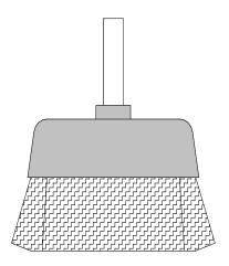
According to above drawing, 2" diameter, 1" trim length. Total  $N^{\circ}$  of .012" wire ends in the brush: 1,600 Weight of total product: 85 gr.
