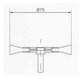
According to above drawing, 3" diameter, Total  $N^{\circ}$  of .012" wire ends in the brush: 2,400 Weight of total product: 98 grs.
